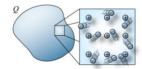
Charges in materials - In solid materials commonly encountered in daily life, positively-charged ions are relatively stuck in place. Some electrons are somewhat looser. Conductors are materials that contain an abundance of electrons that are "very free" to move. **Insulators** are materials that do not contain any electrons that are "very free" to move.
