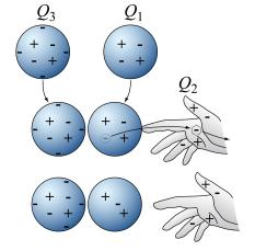
Transfer of charge by friction – transfer of electrons through scraping from one object to another object that more easily grabs onto electrons
